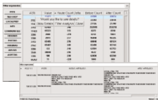
RIB Filter Analysis allows you to drill down to see each of the individual route changes
